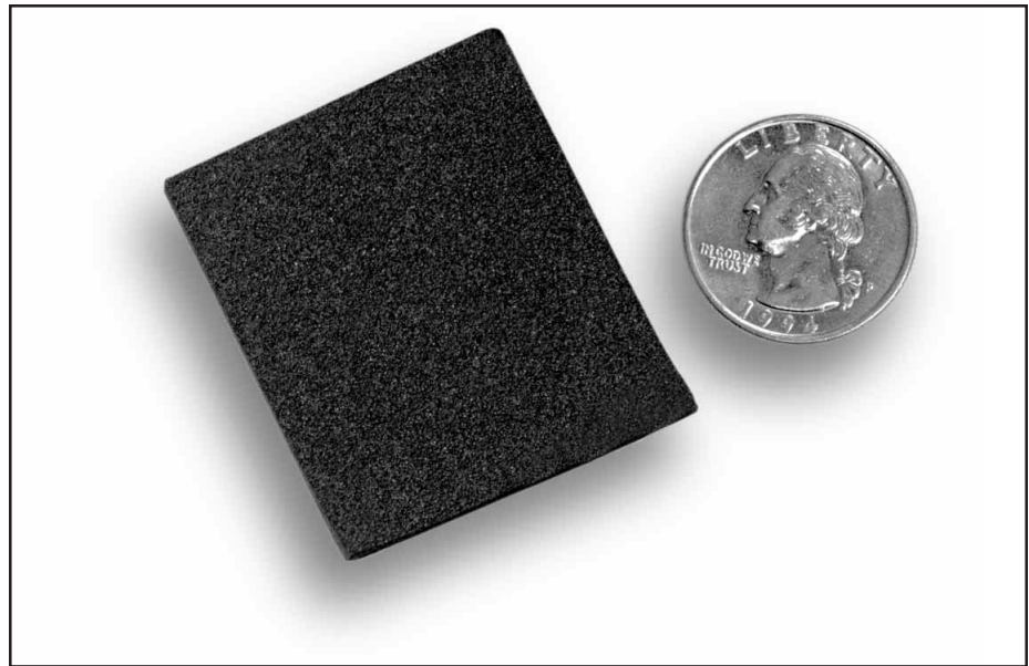
Figure 8. The solution: A neoprene gasket used to seal ventilation holes in the CFL fixtures
