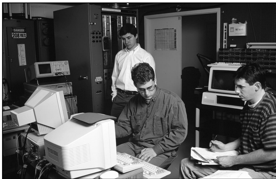
Two students from North Carolina State University (sitting) test the reaction of a local area network (LAN) to sags, surges, and electrical fast transients in the PEAC laboratory. PEAC engineer Doni Nastasi watches the computer monitors as the LAN is subjected to a Ring Wave surge. Results of these tests will be used in phase two of the PC project, which will investigate the immunity and emissions of a typical computer network.
