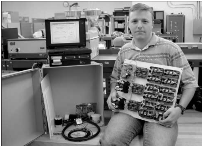
Thomas Cooke, a PEAC laboratory technician, displays the circuit board for the Process Ride-Through Evaluation System, or porto-sag, now available to qualified EPRI-member utilities. The main components of the porto-sag consist of heavy-duty transistors, gate-driver circuits, contact relays, a data-acquisition module, and a laptop computer. External variable transformers, one for each phase of equipment voltage, control the depth of the sag delivered to the equipment.
