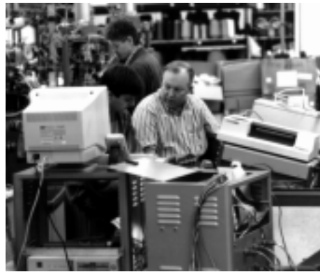
Working in a textile plant, Larry Morgan of Duke Power (right) uses a portable sag generator to investigate power quality problems in a knitting machine.
