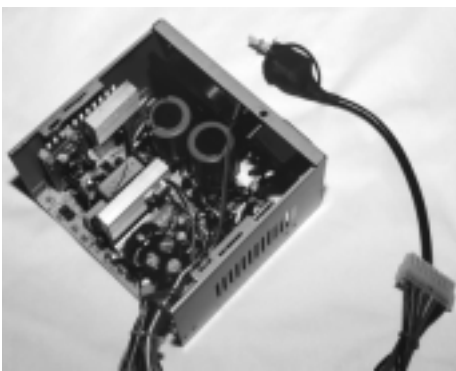
PEAC tests PC power supplies to confirm that off-the-shelf capacitor technology can enable power supplies to ride through voltage sags and interruptions lasting as long as one-half second.
