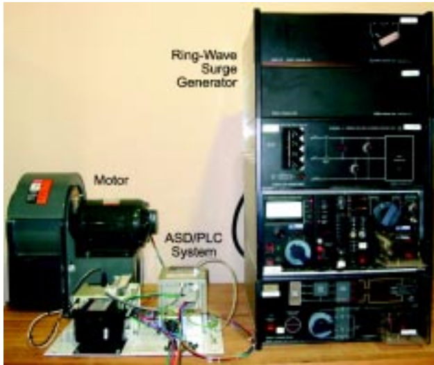
Fig. 3. Test setup for surge testing the communication port of a motor and control system.
